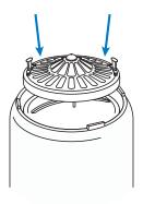
2. Reattach top tank snap ring. Pull up on the top cap to seat the O-rings.
