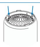
2. Remove the top tank snap ring. Remove the top cap from the housing assembly. Pull the cap out of the top of the tank by lifting up on the handles.
